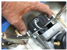
Step 5 • Loosen all 4 nuts on mounts. Hold down on front isolators while lifting front of motor.
