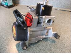
Step 1 • Place supplied rubber isolators on motor mounts.
