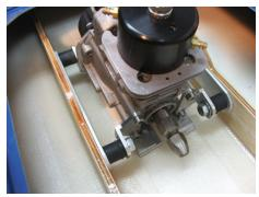
Step 3 • Place motor between rails and shim to your desired position.
