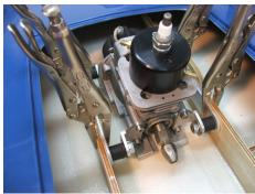
Step 4 • Firmly clamp drill plates to rails as shown. Note: 6" Needle Nose Vise Grips work best.
