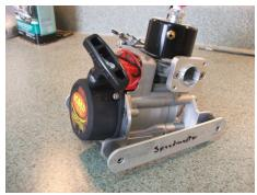
Step 2 • Place drill plates on both sides of motor.
